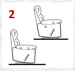
For a stronger backward swinging motion, adjust the height of the front legs.
